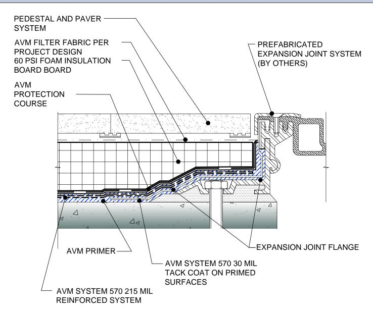
NOTE: AVM PRODUCTS ARE NOT DESIGNED TO WATERPROOF EXPANSION JOINTS. EXPANSION JOINTS REQUIRE A PROPER EXPANSION JOINT MATERIAL MANUFACTURED BY OTHERS. AVM PRODUCTS CAN BE INSTALLED OVER EXPANSION JOINT MATERIALS AS ILLUSTRATED ABOVE. CHECK WITH THE EXPANSION JOINT PRODUCT MANUFACTURER FOR MATERIAL COMPATIBILITY.
