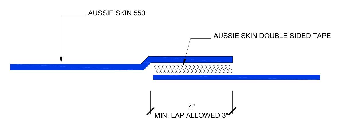
Important Note: When installing the "Non-Factory Lap", The Installation procedure should be as follows:
