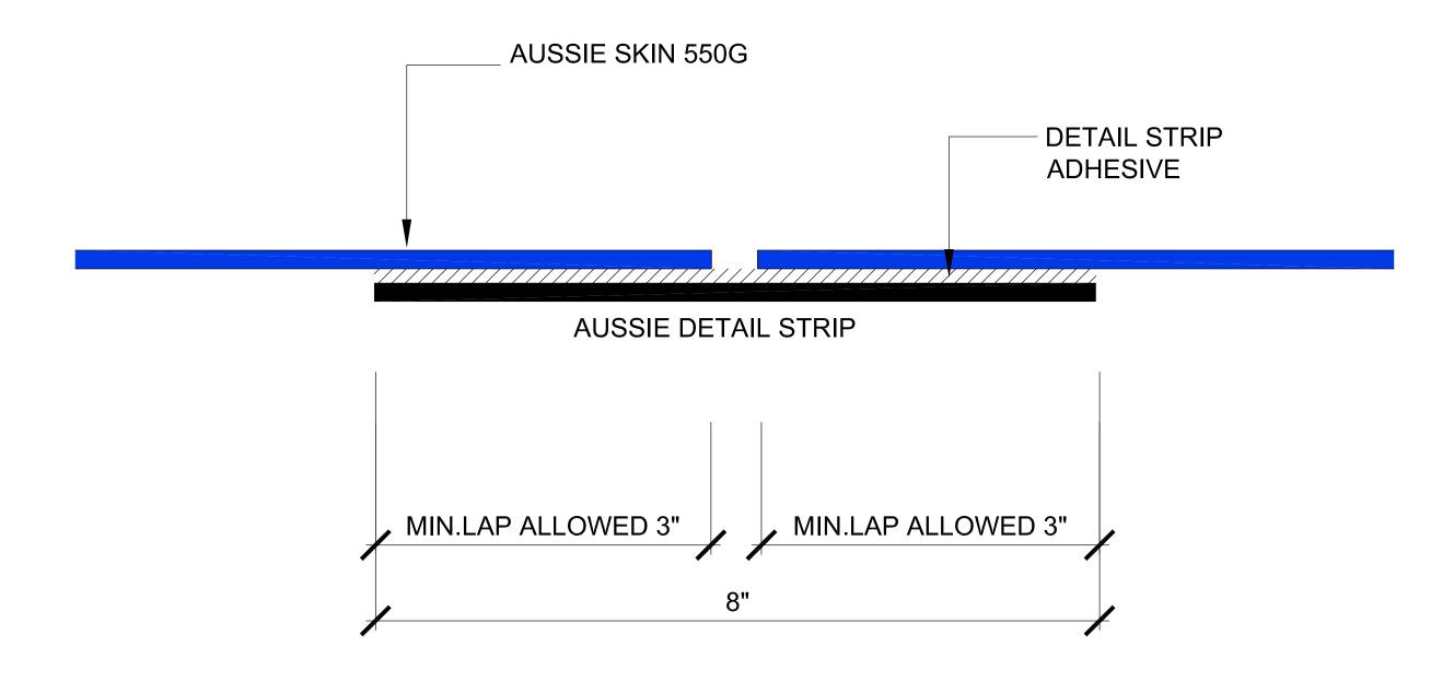
Important Note: When installing the "Alternative Non-Factory Lap", The Installation procedure should be as follows:
