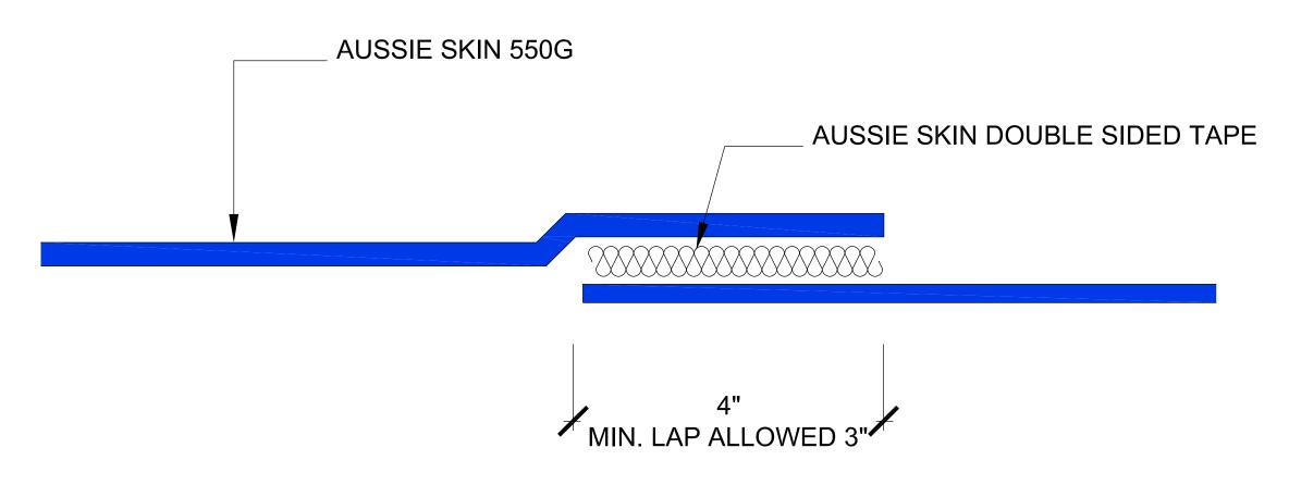
Important Note: When installing the "Non-Factory Lap", The Installation procedure should be as follows:
