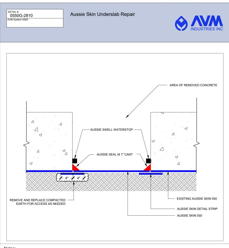
1. Aussie Skin 550 is a Heavy, Duty, Easy to Install, Puncture Resistant Sheet Waterproofing Membrane with added technologies creating excellent adhesion between the membrane and wet Concrete or Shot-Crete.
