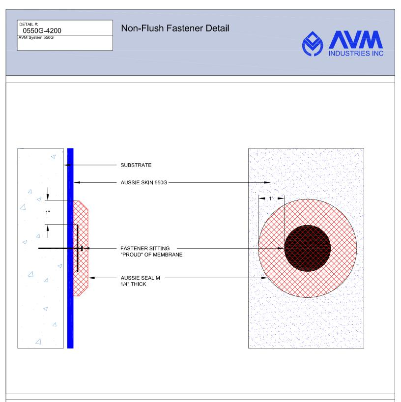
1. Aussie Skin 550G is a Heavy, Duty, Easy to Install, Puncture Resistant Sheet Waterproofing Membrane with added technologies creating excellent adhesion between the membrane and wet Concrete or Shot-Crete.
