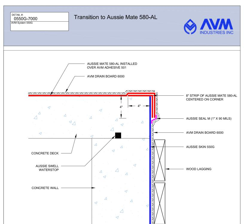
1. Aussie Skin 550G is a Heavy, Duty, Easy to Install, Puncture Resistant Sheet Waterproofing Membrane with added technologies creating excellent adhesion between the membrane and wet Concrete or Shot-Crete.
