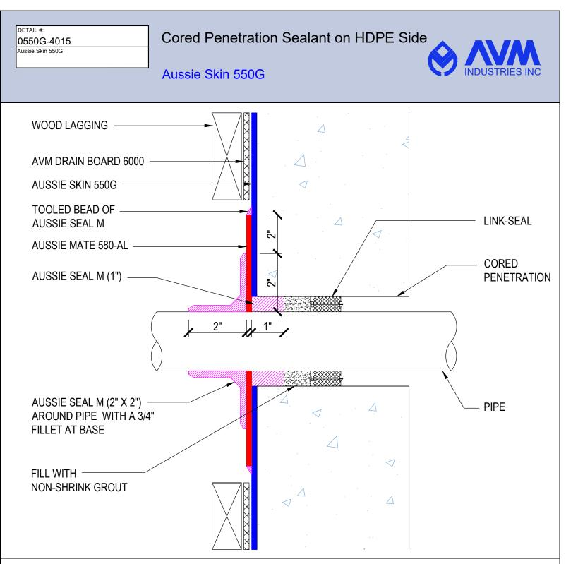
1. Aussie Skin 550G is a Heavy, Duty, Easy to Install, Puncture Resistant Sheet Waterproofing Membrane with added technologies creating excellent adhesion between the membrane and wet Concrete or Shot-Crete. Creating excellent adhesion between the membrane and wet Concrete or Shot-Crete.
