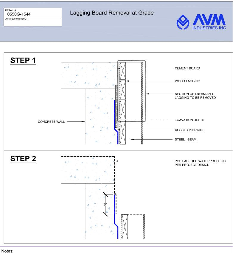
1. Aussie Skin 550G is a Heavy, Duty, Easy to Install, Puncture Resistant Sheet Waterproofing Membrane with added technologies creating excellent adhesion between the membrane and wet Concrete or Shot-Crete.
