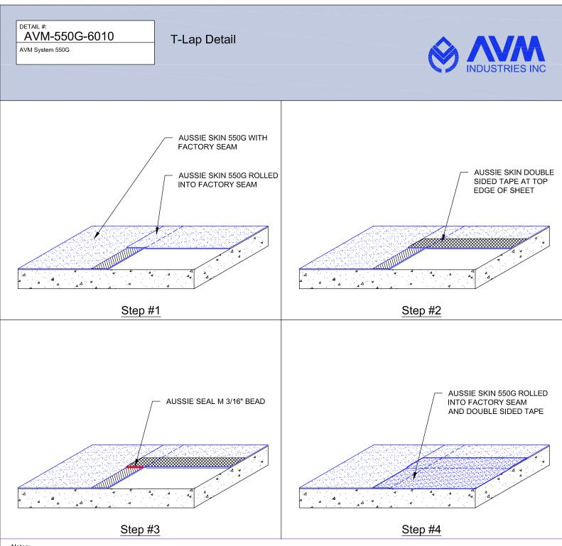
1. Aussie Skin 550G is a Heavy, Duty, Easy to Install, Puncture Resistant Sheet Waterproofing Membrane with added technologies creating excellent adhesion between the membrane and wet Concrete or Shot-Crete.
