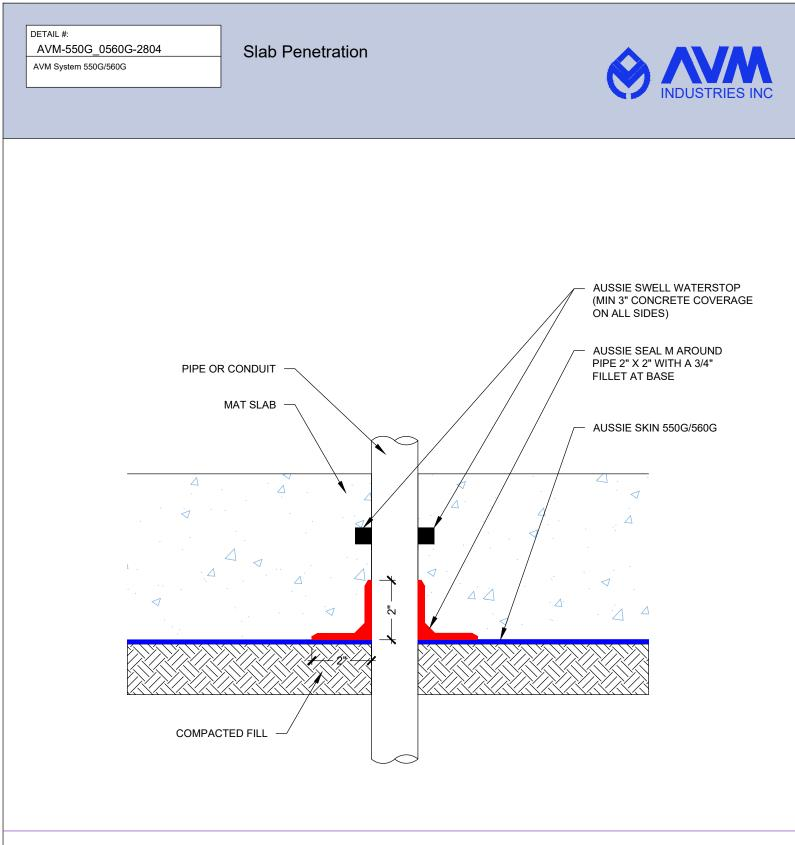
Aussie Skin 550G and 560G are Heavy Duty, Easy to Install, Puncture Resistant Sheet Waterproofing Membranes with added technologies creating excellent adhesion between the membrane and wet Concrete or Shotcrete. Aussie Skin 560G is an approved methane/VOC barrier.
