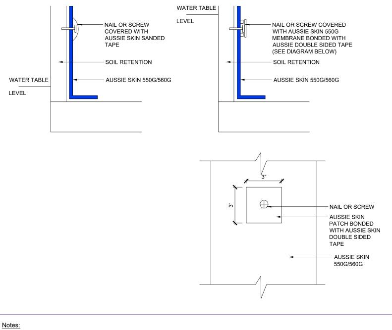
1. Aussie Skin 550G and 560G are Heavy Duty, Easy to Install, Puncture Resistant Sheet Waterproofing Membranes with added technologies creating excellent adhesion between the membrane and wet Concrete or Shotcrete. Aussie Skin 560G is an approved methane/VOC barrier.
