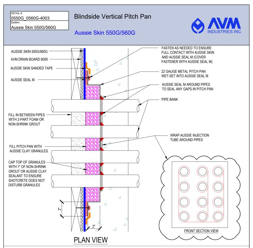
1. Aussie Skin 550G and 560G are Heavy Duty, Easy to Install, Puncture Resistant Sheet Waterproofing Membranes with added technologies creating excellent adhesion between the membrane and wet Concrete or Shotcrete. Aussie Skin 560G is an approved methane/VOC barrier.
