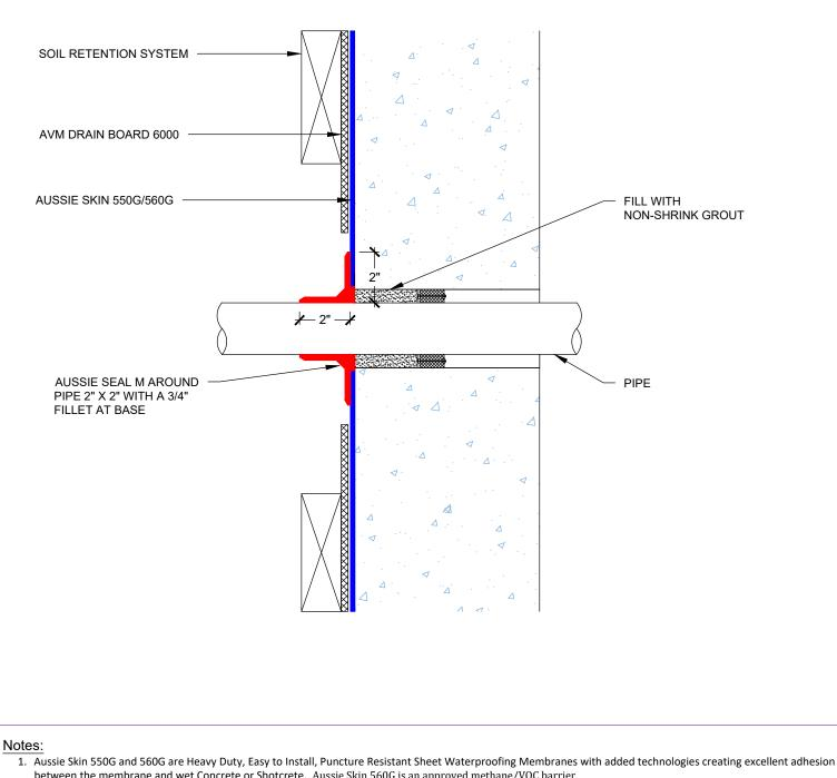
between the membrane and wet Concrete or Shotcrete. Aussie Skin 560G is an approved methane/VOC barrier.
