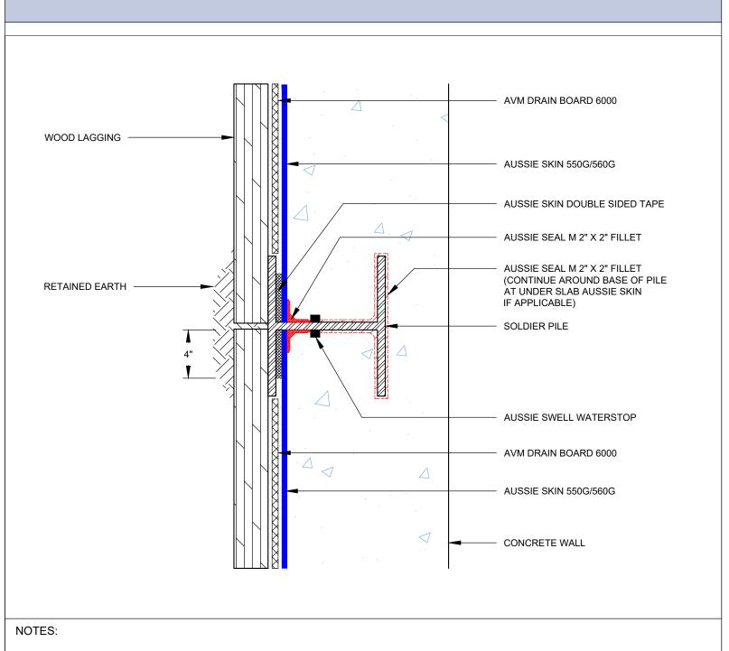
Aussie Skin 550G and 560G are Heavy Duty, Easy to Install, Puncture Resistant Sheet Waterproofing Membranes with added technologies creating excellent adhesion between the membrane and wet Concrete or Shotcrete. Aussie Skin 560G is an approved methane/VOC barrier.
