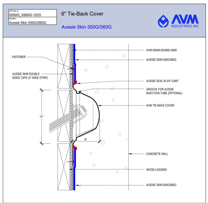
1. Aussie Skin 550G and 560G are Heavy Duty, Easy to Install, Puncture Resistant Sheet Waterproofing Membranes with added technologies creating excellent adhesion between the membrane and wet Concrete or Shotcrete. Aussie Skin 560G is an approved methane/VOC barrier.
