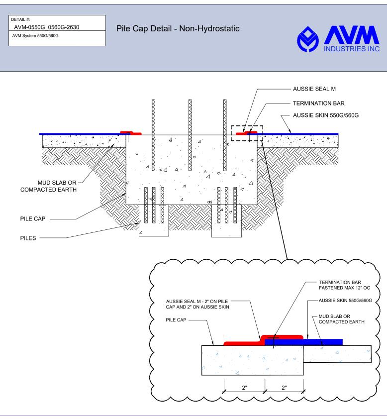
1. Aussie Skin 550G and 560G are Heavy Duty, Easy to Install, Puncture Resistant Sheet Waterproofing Membranes with added technologies creating excellent adhesion between the membrane and wet Concrete or Shotcrete. Aussie Skin 560G is an approved methane/VOC barrier.
