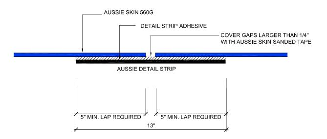
Important Note: When installing the "Alternative Non-Factory Lap", The Installation procedure should be as follows:
