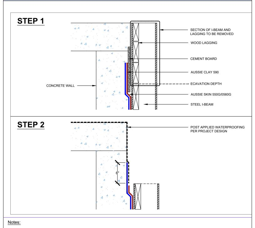
1. Aussie Clay & Aussie Clay PL are bentonite sheet membranes for waterproofing below-grade vertical and horizontal surfaces, including blindside and backfilled applications. Aussie Clay can be used with shotcrete or cast in place concrete in hydrostatic or non-hydrostatic conditions.
