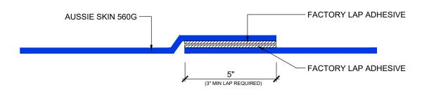
Important Note: When installing the "Factory Lap", The Installation procedure should be as follows:
