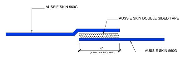
Important Note: When installing the "Non-Factory Lap", The Installation procedure should be as follows:
