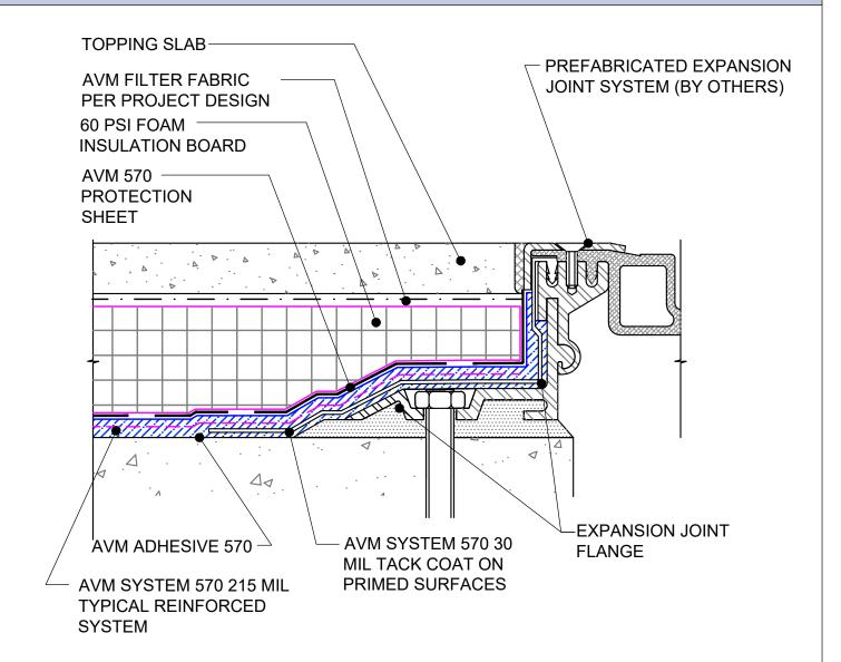
NOTE: AVM PRODUCTS ARE NOT DESIGNED TO WATERPROOF EXPANSION JOINTS. EXPANSION JOINTS REQUIRE A PROPER EXPANSION JOINT MATERIAL MANUFACTURED BY OTHERS. AVM PRODUCTS CAN BE INSTALLED OVER EXPANSION JOINT MATERIALS AS ILLUSTRATED ABOVE. CHECK WITH THE EXPANSION JOINT PRODUCT MANUFACTURER FOR MATERIAL COMPATIBILITY.
