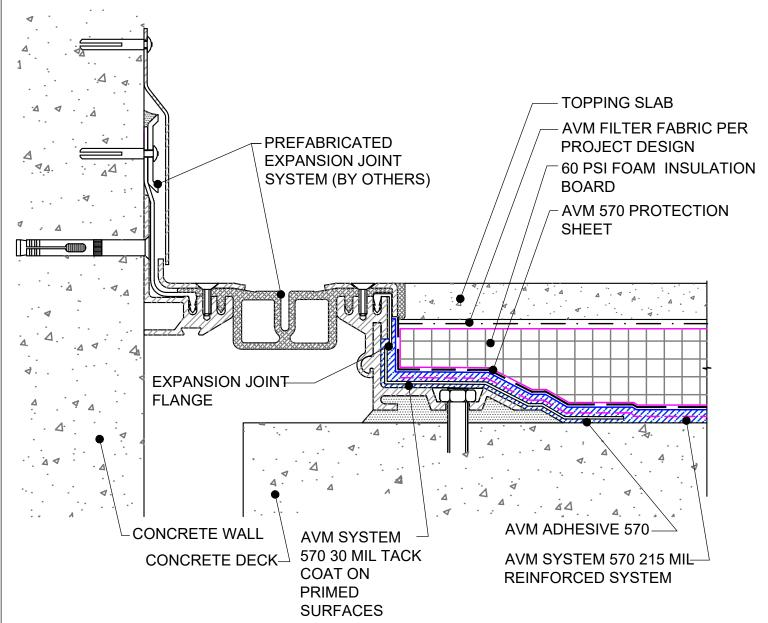
NOTE: AVM PRODUCTS ARE NOT DESIGNED TO WATERPROOF EXPANSION JOINTS. EXPANSION JOINTS REQUIRE A PROPER EXPANSION JOINT MATERIAL MANUFACTURED BY OTHERS. AVM PRODUCTS CAN BE INSTALLED OVER EXPANSION JOINT MATERIALS AS ILLUSTRATED ABOVE. CHECK WITH THE EXPANSION JOINT PRODUCT MANUFACTURER FOR MATERIAL COMPATIBILITY.
