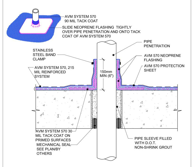
NOTE: CLEAN ALL PENETRATIONS OF DIRT, RUST AND OIL. ROUGHEN SURFACE OF PIPE BEFORE APPLYING PRIMER. VERIFY PENETRATION IS PROPERLY SECURED TO DECK OR WALL TO AVOID MOVEMENT OF PIPE.
