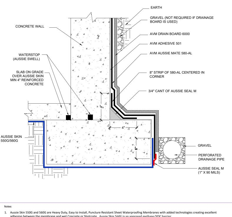
adhesion between the membrane and wet Concrete or Shotcrete. Aussie Skin 560G is an approved methane/VOC barrier.
