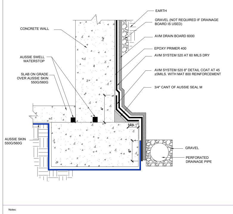
1. Aussie Skin 550G and 560G are Heavy Duty, Easy to Install, Puncture Resistant Sheet Waterproofing Membranes with added technologies creating excellent adhesion between the membrane and wet Concrete or Shotcrete. Aussie Skin 560G is an approved methane/VOC barrier.
