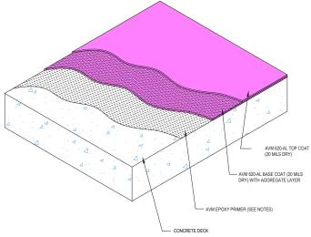
FIGURE 2.2 - TYPICAL ASSEMBLY OVER CONCRETE
