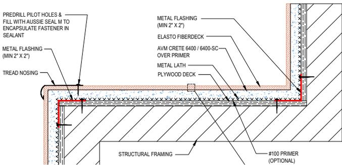
The threshold detail is going to be similar to the installation over concrete substrates but with the addition of the Metal Lath and AVM Crete 6400 as shown as follows.
