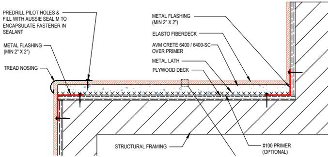
For installation of stairs over plywood where there is tread and riser, the AVM Crete 6400 would be installed over both the horizontal and vertical portions of the stairs. See below diagram.
