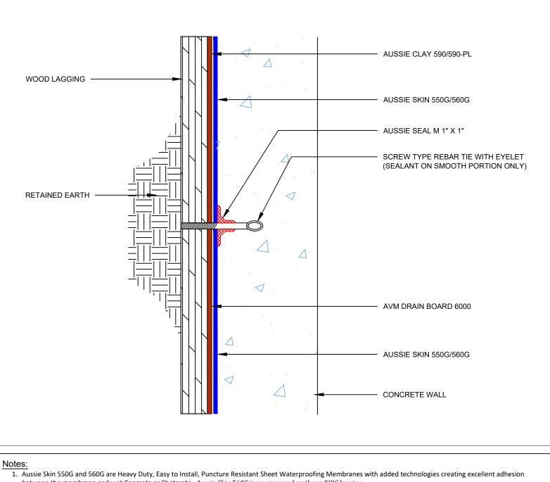
between the membrane and wet Concrete or Shotcrete. Aussie Skin 560G is an approved methane/VOC barrier.
